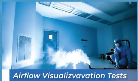
Airflow Visualizavation Tests
